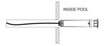
2) Insert the ColorLogic/CrystaLogic 1.5" LED light fully into the conduit. Insert the included hex nut tool into the 3 slots on the light face as shown.
