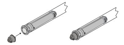
3) Slide the ring tool over the nut tool and insert tabs into the light face. Hold the nut tool with a wrench while rotating the ring tool clockwise. Handtighten the ring tool until snug. Do not overtighen.
