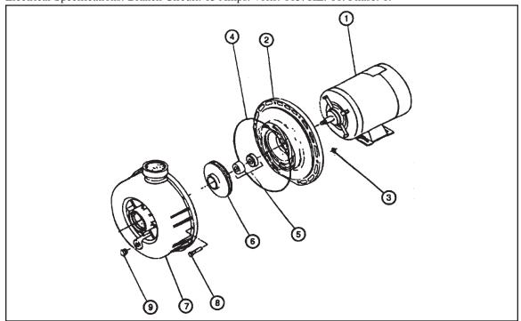
Dynamo Pump Replacement Parts for Predator II System
