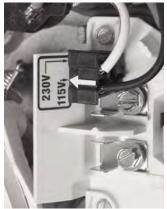
Figure 4A -Voltage Change Plug Set for 230 Volts
