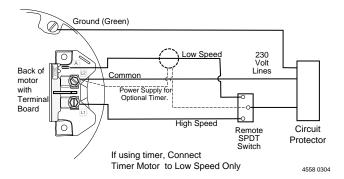
Minimum switch and timer amp rating must equal Branch Fuse Rating given in "Recommended Fusing and Wiring Data" table.
