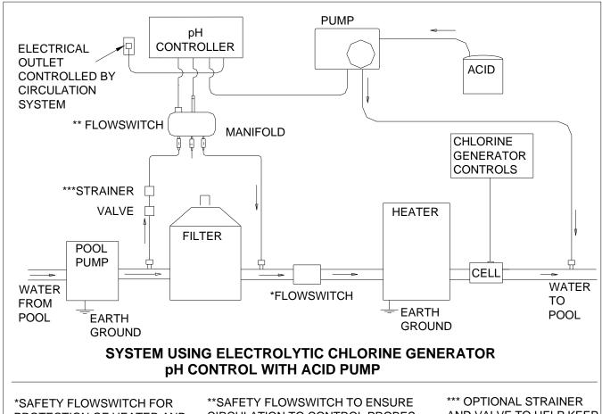
\*SAFETY FLOWSWITCH FOR PROTECTION OF HEATER AND TO ENSURE DILUTION OF CHEMICAL INTO POOL. \*\*SAFETY FLOWSWITCH TO ENSURE CIRCULATION TO CONTROL PROBES AND INDICATOR THAT POOL CIRCULATION IS OCCURRING.
