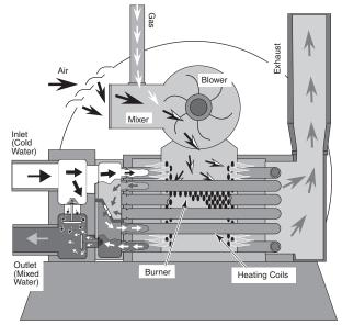
An electronic temperature sensing **thermistor** in the manifold adapter inlet controls the heater operation. When the inlet water
