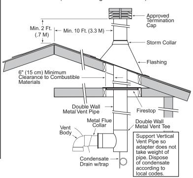
**Figure 18. –** Typical Metal Vent Pipe Installation -Canada (Vertical – Negative Pressure)
