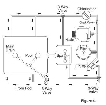
*NOTICE:* If the heater is plumbed in backwards, it will cycle continuously. Make sure piping from filter is not reversed when installing heater.
