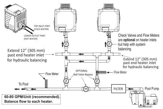
Figure 5. Two MasterTemp® Heaters Plumbing Hydraulic Diagram
