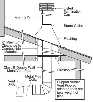
Figure 17. – Typical Metal Vent Pipe Installation - U.S. (Vertical – Negative Pressure)
