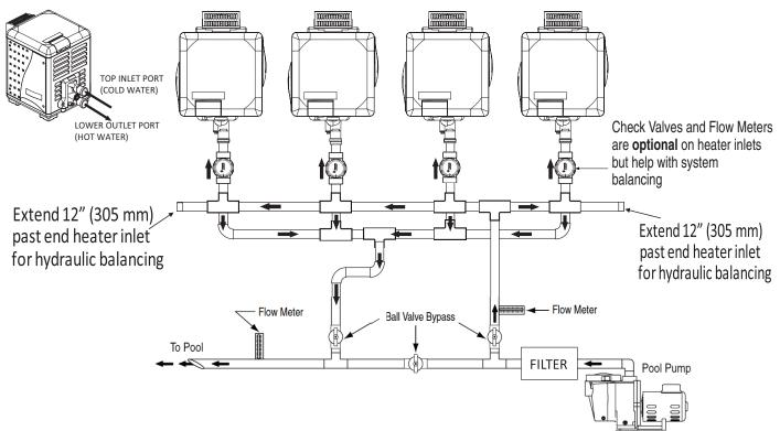
Figure 6. Four MasterTemp Heaters Plumbing Hydraulic Diagram
