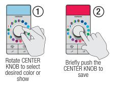
If you try to save the same color or show that is currently selected, the Light Controller will indicate that no change will occur by blinking LED 1 (see LED Indicator Codes) and remain in Show/Color mode
