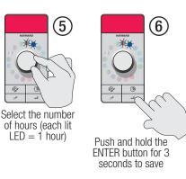
The Light Controller will indicate that a new schedule has been set by blinking LED 4 (see LED Indicator Codes) and then revert to Show/Color mode.
