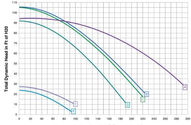
Volumetric Flow Rate in US Gallons Per Minute
