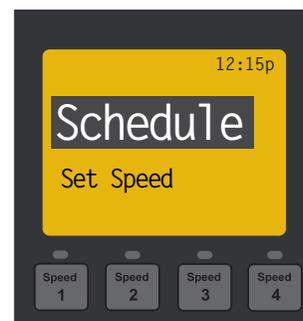
The pump will prime and begin to run the programmed schedule at the specified start time. When running in Schedule or Egg Timer mode, the countdown time (T 00:01) showing the hours and minutes remaining is displayed.
