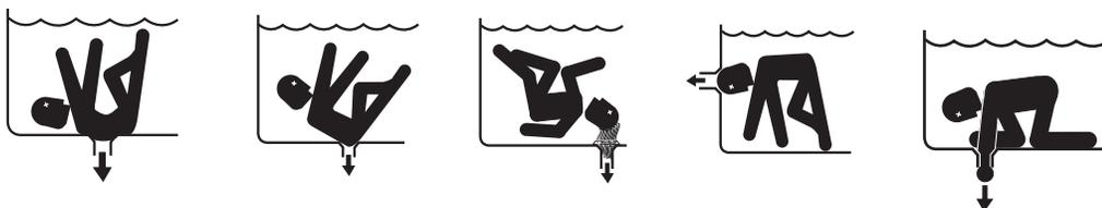
THIS PUMP PRODUCES HIGH LEVELS OF SUCTION AND CREATES A STRONG VACUUM AT THE MAIN DRAIN AT THE BOTTOM OF YOUR POOL OR SPA. THIS SUCTION IS SO STRONG THAT IT CAN TRAP ADULTS OR CHILDREN UNDER WATER IF THEY COME IN CLOSE PROXIMITY TO A POOL OR SPA DRAIN OR A LOOSE OR BROKEN DRAIN COVER OR GRATE.
