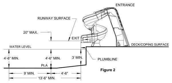
2. A minimum clearance area in front of the slide shall be maintained at all times as follows:
