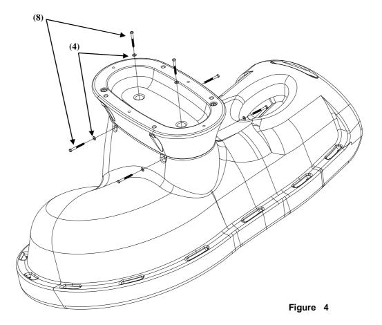
3) Place the assembled runway exit section and pedestal upright so that the pedestal is resting on the ground. Notes: It may take more than one person to perform this step. Verify that the gasket material is properly attached before assembling the parts.
